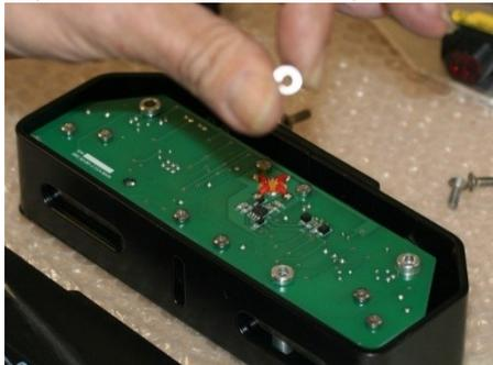
8. Put the cover back on the Copycounter, align the holes in the cover, spacers and PCB then screw the M4 countersunk screws back.
