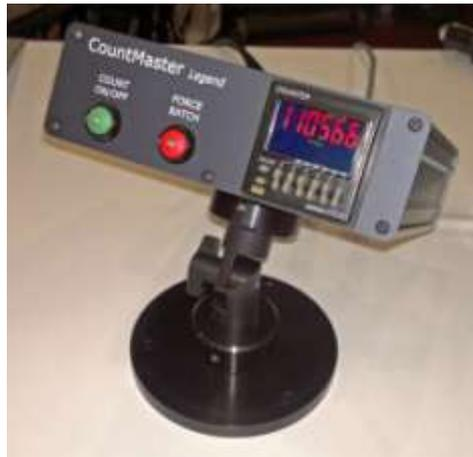
The CountMaster Legend is an industrial totalizer and batch counter with a batch signal output configurable to drive 120VAC (USA only), 24VDC or volt-free contacts to activate batching devices. The count input signal is configurable as NPN (sink), PNP (source) or "totem pole" to accommodate any standard sensor. For easy installation talk to our sales team and they will configure the CountMaster to your requirements before shipping.
